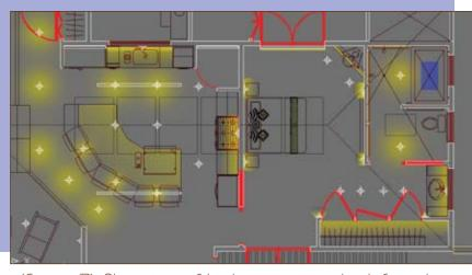
(Figure 7) Plan view of kitchen area on the left and master bedroom on the right, with lighting zones highlighted in yellow.
