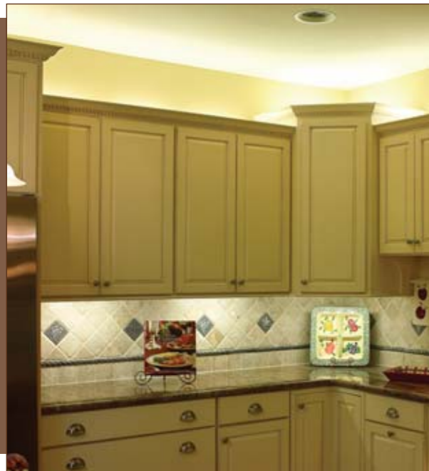
(Figure 2) Linear fluorescent lights above and below cabinets fill in shadows and increase the impression of brightness while producing a glare-free environment.
