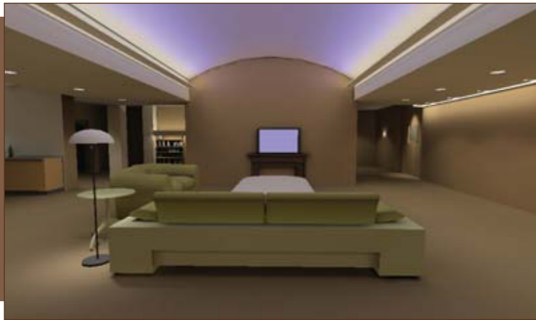
(Figure 6) Great Room Color-changing LED system is concealed in cove along each side of great room to uplift vaulted ceiling, and provide mood and circadian benefits; blue light has been found to be effective in activating the circadian system.
