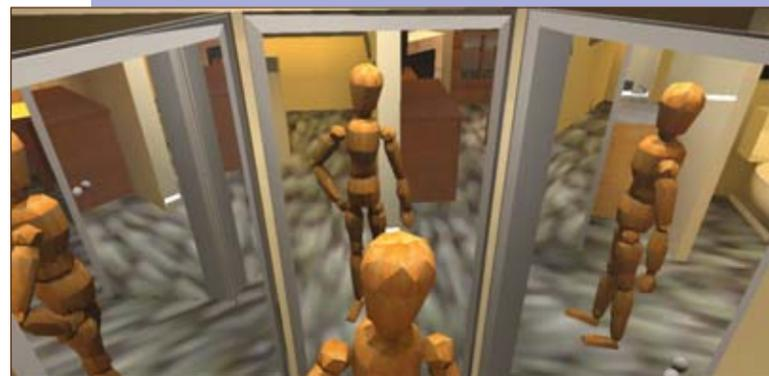
(Figure 8) In an area that acts as a fitting room, providing multiple lighting conditions allow the homeowners to see how they would look in different environments. Here, both high-color rendering and cool-color temperature fluorescent track heads contrast with warm halogen track heads. The track system accommodates both, so either or both can be used at one time; track heads shown are by Lightolier ([www.lightolier.com](http://www.lightolier.com)).
